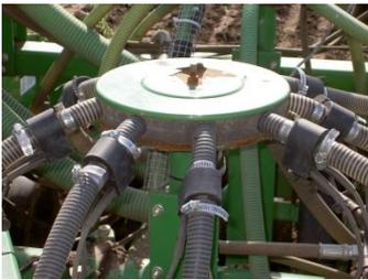
1. Select a mounting location near the distributor. The Sensor Loop Cables should not be stretched tight when connected.
